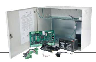
The PW6K1OUT interfaces with the intelligent control module (PW6K1IC or PW3K1IC) providing up to 16-relay output control —12 relays on the front edge. Relays may be used for elevator control, status annunciation and for general facility control, such as door monitoring.
